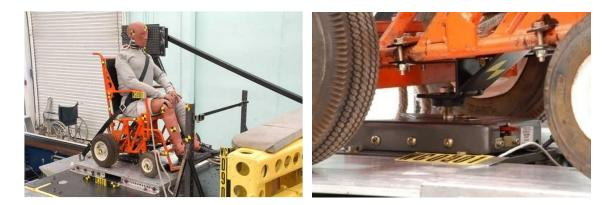
Figure 4-1. Sled test setup (Left) and the single point docking system (Right).
