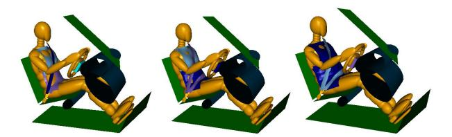
Figure 3-3. Modified Torso Model with BMIs of 25 (Left), 30 (Middle) and 39 (Right).
