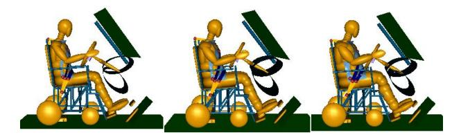
Figure 4-7. The Obese Wheelchair-seated Occupant Model with BMIs of 25 (Left), 30 (Middle), and 39 (Right).
