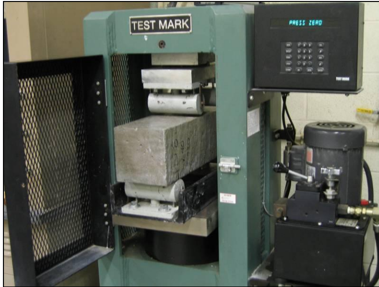
Figure C 6. Flexural strength test setup.
