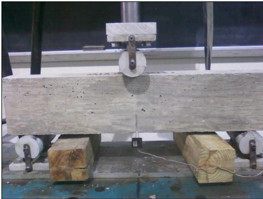
Figure C 5. Fracture energy test in progress.
