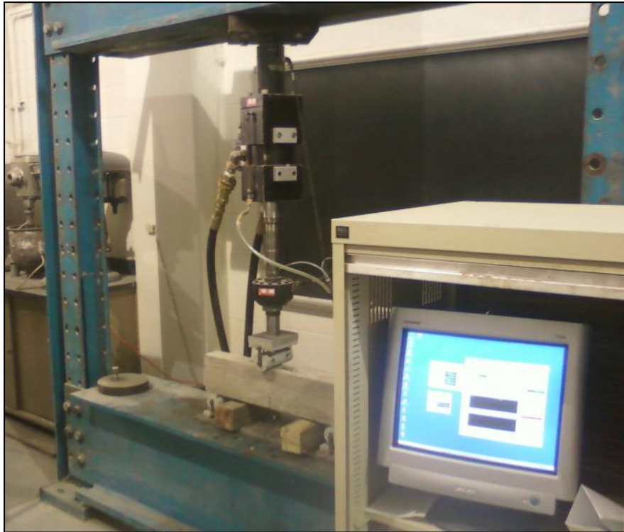
Figure C 1. Fracture energy test setup.
