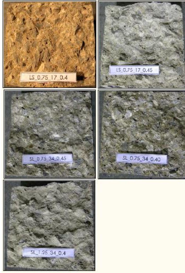
Figure 20. Samples of fractured surfaces for the five concrete mixtures of the present study.
