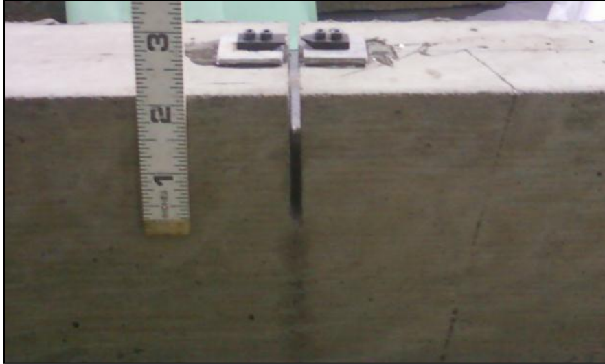
Figure C 4. Saw-cut notch of fracture energy beams.
