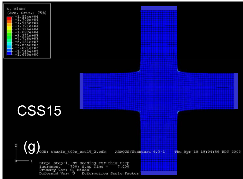
Figure 4-5 a-d) finite element simulation of effects of different gripping methods at 45-degree material axes, e-g) at 0-degree material axes. Plotted in same color scale in each group for easy comparison.
