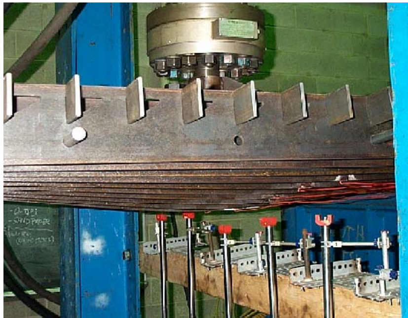
Figure B6 – Transverse Deflection Profile
