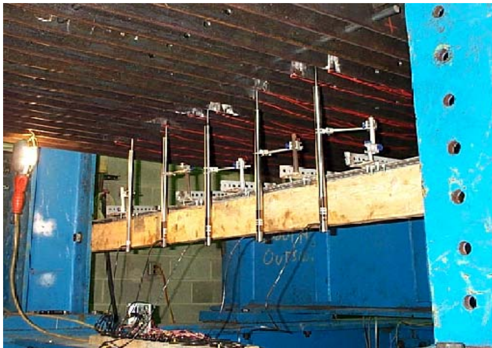
Figure B2 – DCDT Stand and Circuit Board
