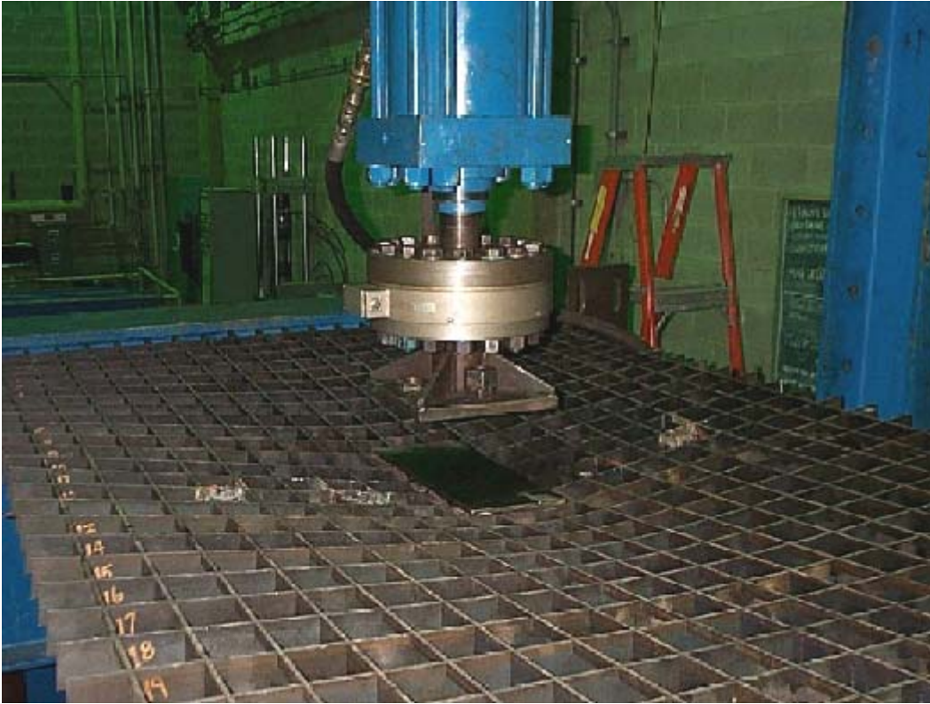
Figure B5 – 250 Kip Actuator and Failed Weldless Grid Deck
