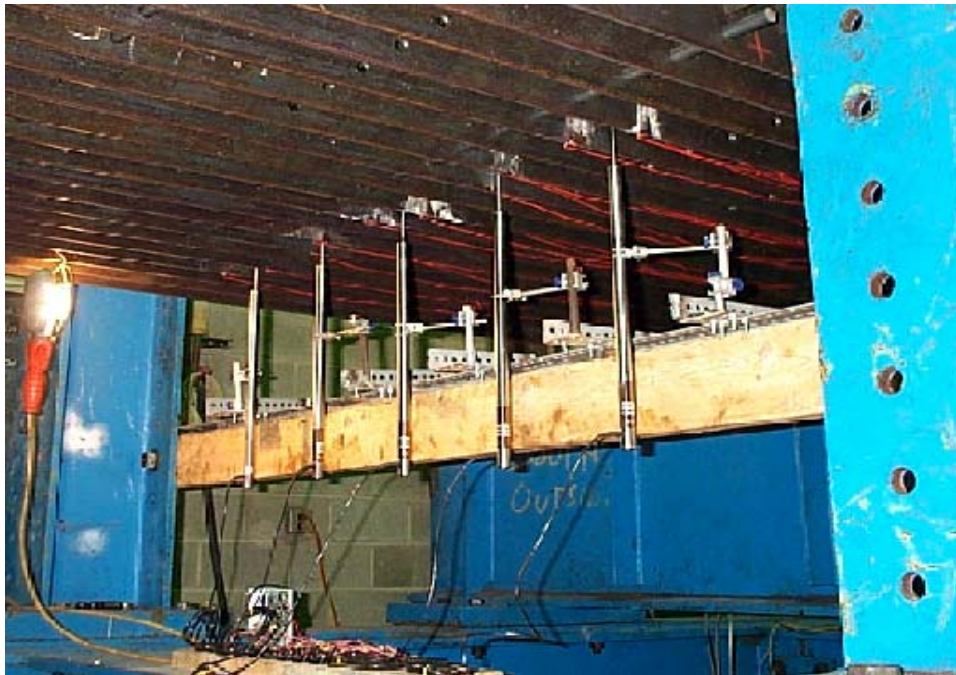
Figure B2 – DCDT Stand and Circuit Board
