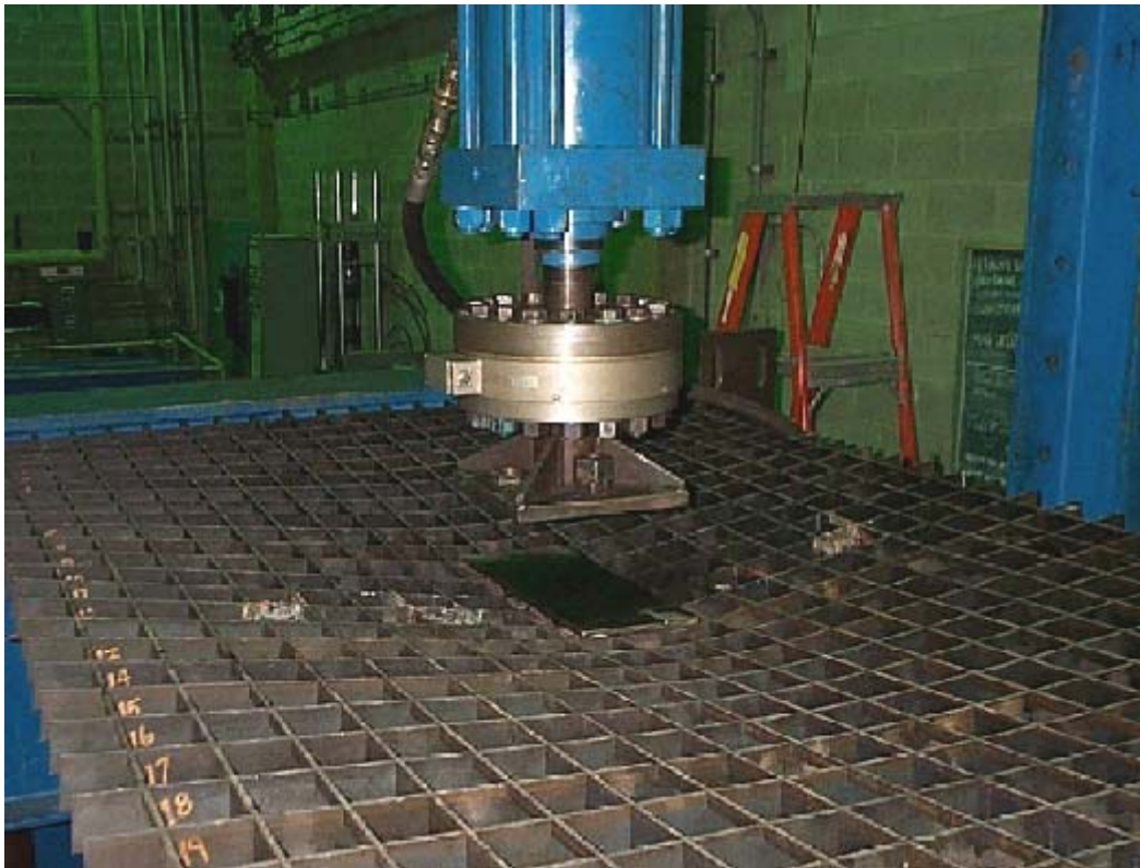
Figure B5 – 250 Kip Actuator and Failed Weldless Grid Deck
