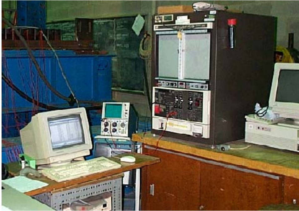
Figure B1 – MTS 458 Controller and Data Acquisition System
