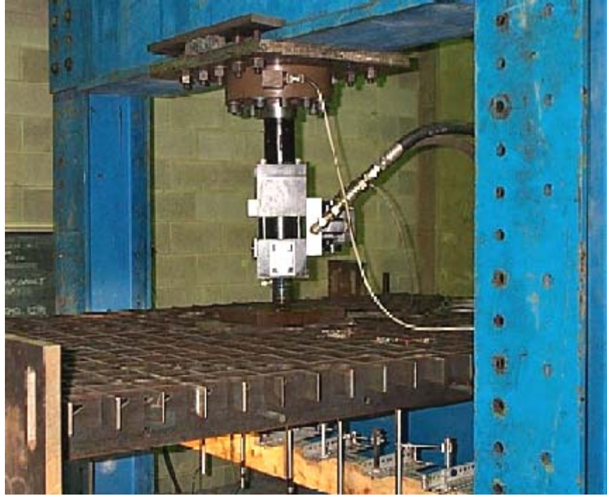
Figure B3 – 25 Kip Actuator Used in Fatigue Testing
