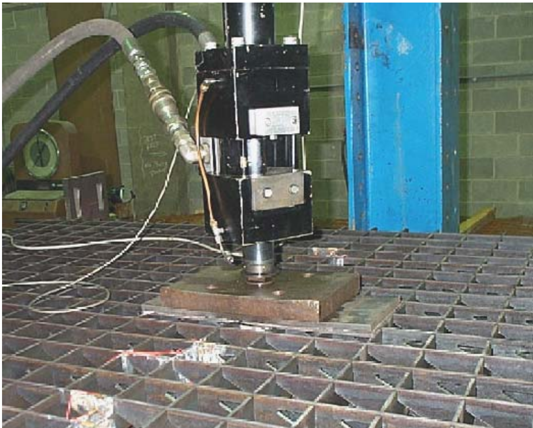
Figure B4 – Foot of Actuator Used in Applying Load
