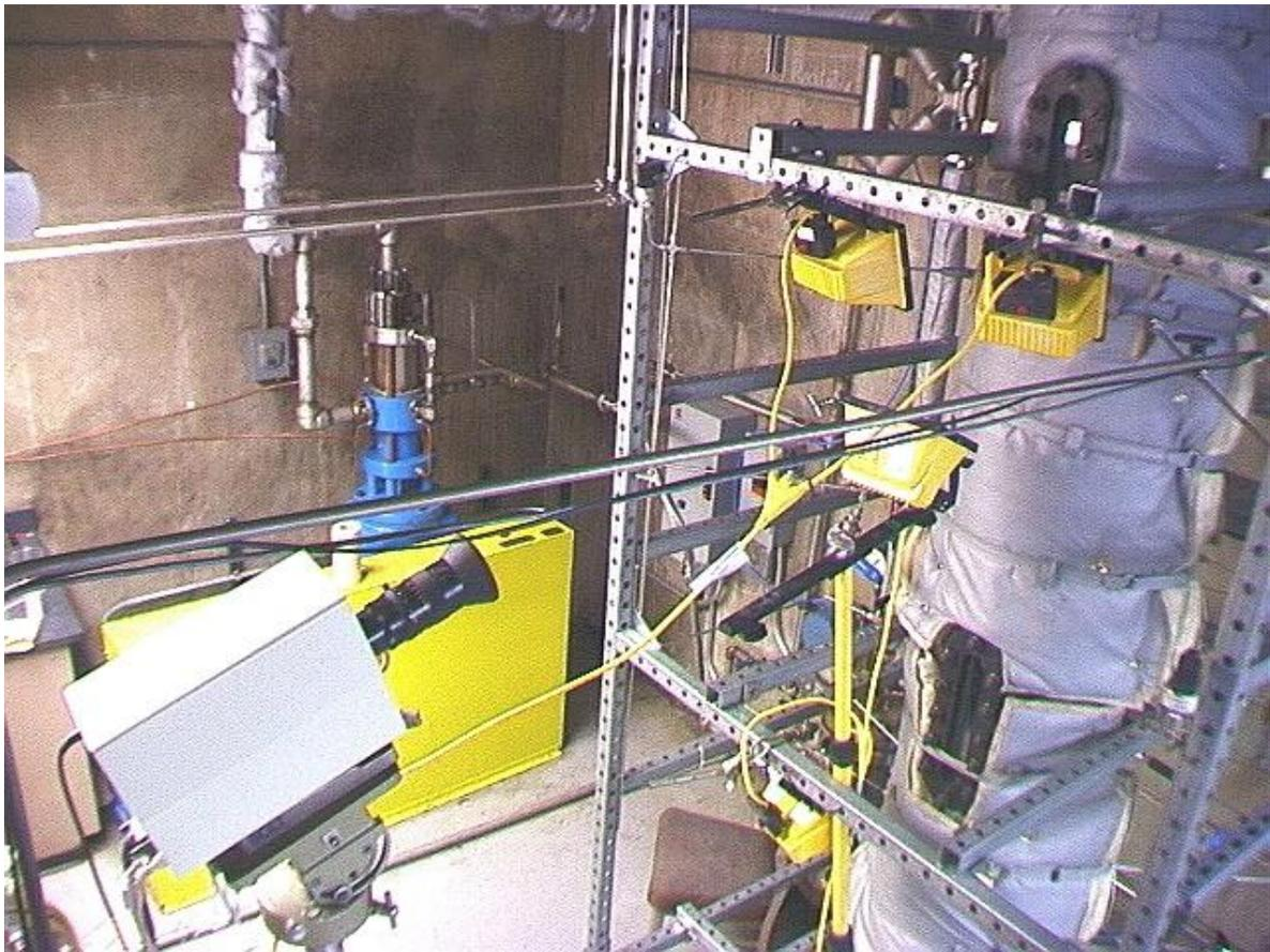
**Figure 22 Picture of the Setup for the High-Speed Phantom Camera used with the Hot SBCR**
