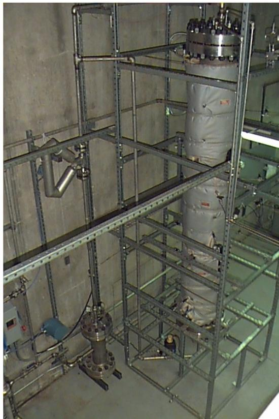
**Figure 19 Pictures of the Hot Slurry Bubble Column Reactor**
