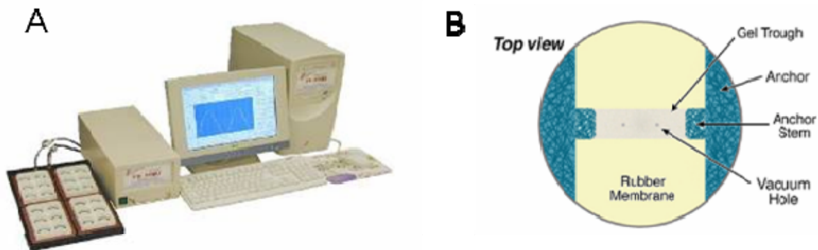
Figure 3-4: (A) Flexcell device and (B) top view of tissue train plate. Figure adapted from www.flexcellint.com .
