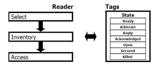
Figure 3 - Interrogator/Tag operations and tag state (EPCglobal Inc., 2008)
