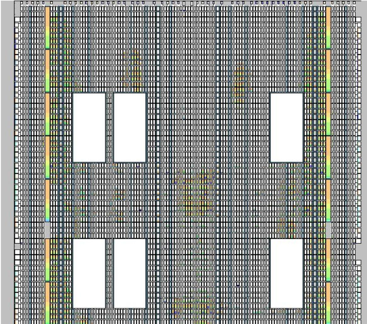
**Figure 38: Post Place and Route Floor Plan of 88 PE (DSP)**
