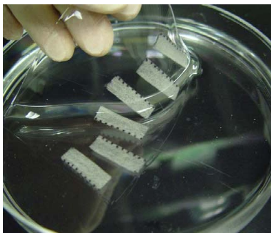
Figure 53 Photograph of polyacrylamide gel-infiltrated scaffold preparation.
