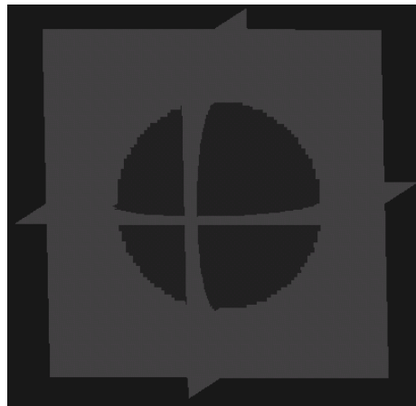
Figure 6 Computer generated 3D data of a sphere of radius 30 voxels, inner intensity of 32, and outer intensity of 64.
