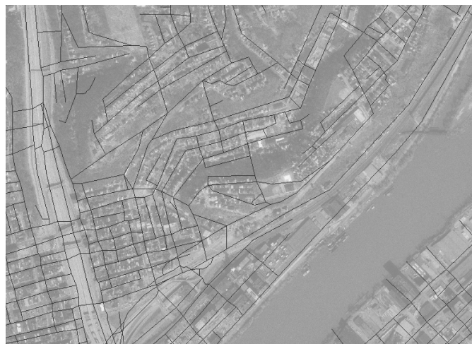
Figure 2.2 A layered map containing both vector objects and raster backdrop 1
