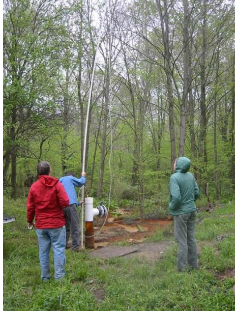
Figure 8. Measuring hydraulic head of monitoring well MW1.
