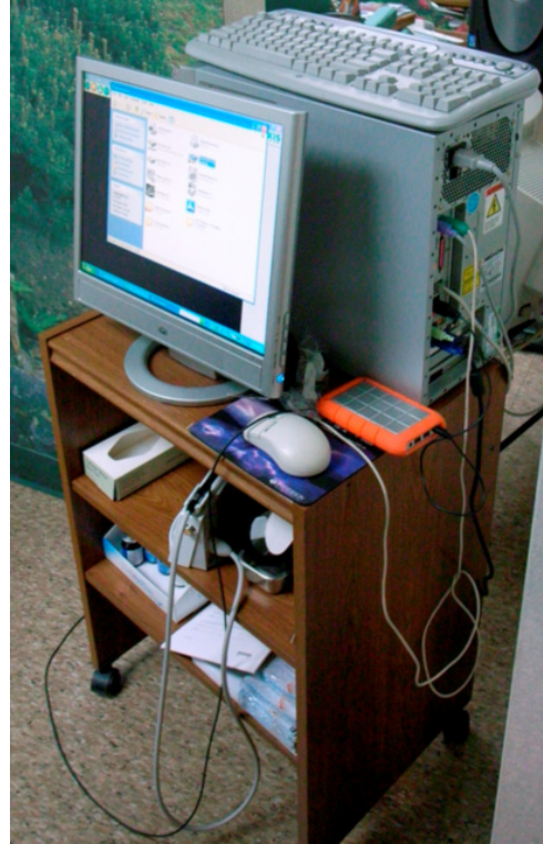
Figure 14. Example of Poor Hardware Integration
