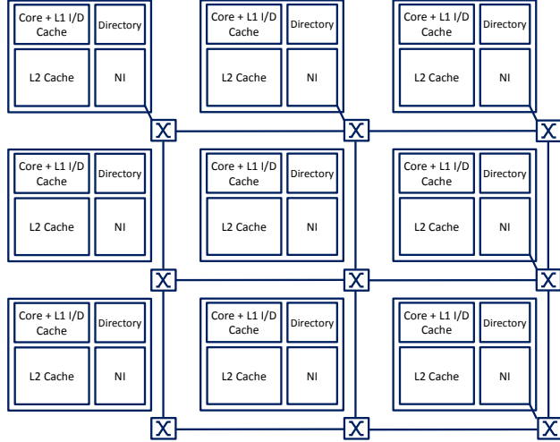
Figure 2: Diagram of a tiled CMP having 9 cores. The tiles are laid out in a 2D mesh. Each tile has a processing core, a private I/D L1 cache, a slice of the L2 cache, a slice of a distributed directory for maintaining cache coherency, and a network interface (NI). Each NI is connected to the router(s) of the interconnect plane(s) at the tile.
