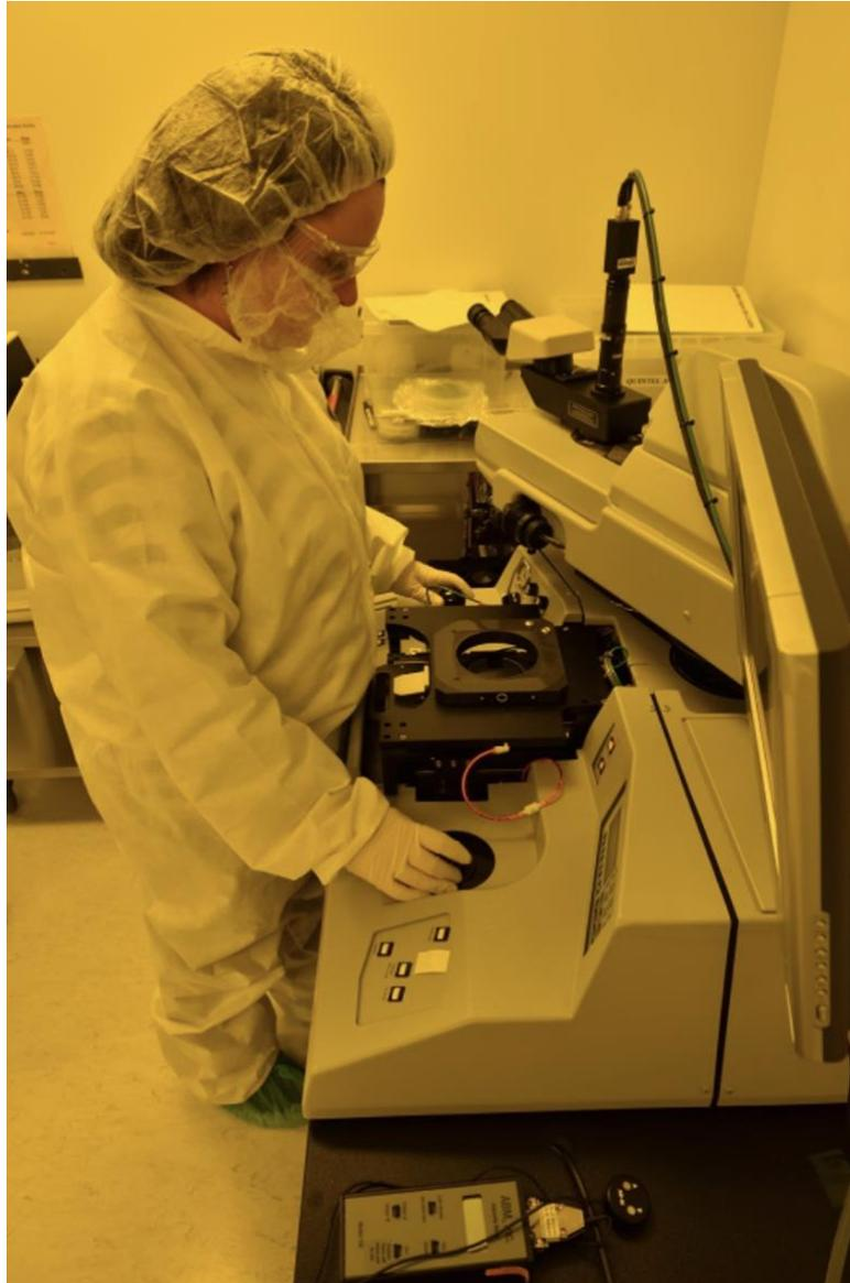
**Figure 8 Quntel Q4000 MA mask aligner located at NFCF at University of Pittsburgh. Picture taken from NFCF webpage.**
