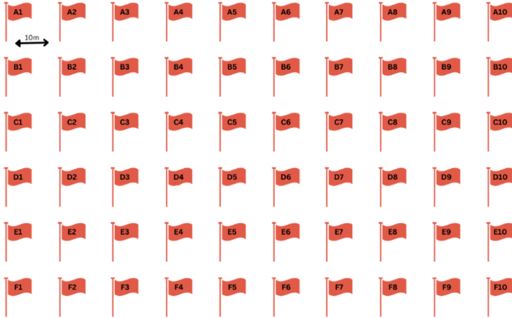
Figure 7. Standard set up of grids. Each grid was set to cover 6000m 2 . The structure of each grid site was set to follow this model unless the landscape prevented the setup. This grid represents the grid at BOM, SGL42, SGL232, and CCH
