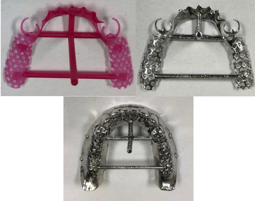
Figure 3: (A)(Left) SLA printed castable resin pattern (B)(Right) After resin being casted with Vitallium 2000 and (C) (Bottom) RPD seated on master model
