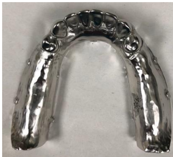
Figure 4: Milled CoCr master model used for mechanical testing.
