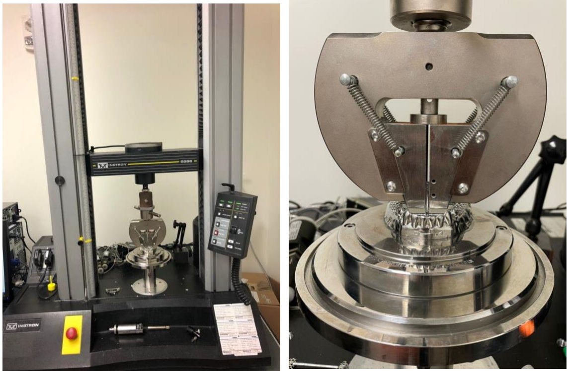
Figure 5 Universal testing machine (Instron) with master model and sample mounted.
