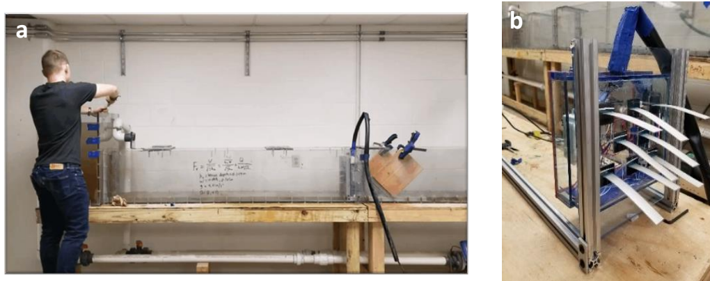
Figure 16: The experimental setup for the wave tank for demonstrating the direct wave piezoelectric energy harvester model; a) the wave tank and the positioning of the piezoelectric elements are shown and b) the support that contains the array of piezoelectric strips are shown in a close-up.
