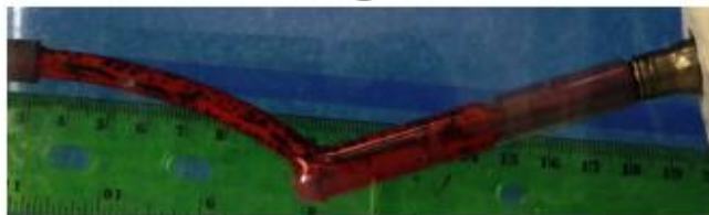
Figure 5.27 a. Pressure-volume and end displacement-volume relations for a tube where an instability was triggered inside a 10.2mm limiter and propagated past the limiter's exit. b. Setup with a 10.2mm limiter that covers part of the tube. c. Initiation of bulge within limiter. d. Bulge exiting limiter.
