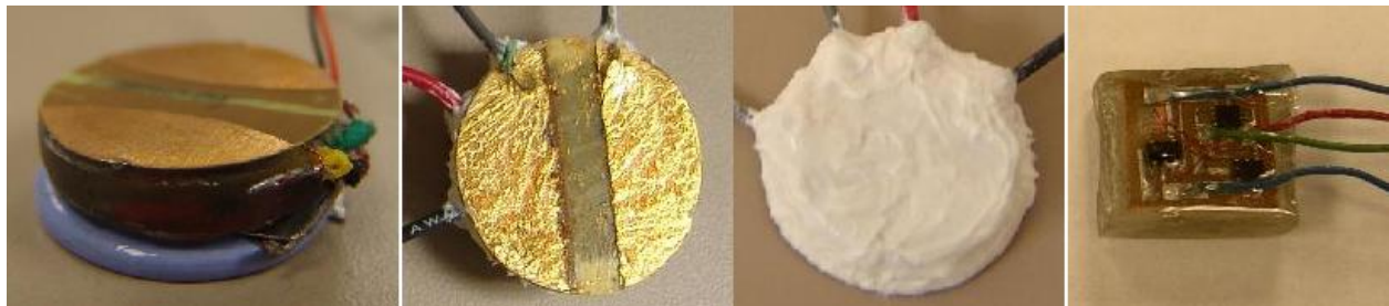
Figure 3.9: Left: First generation of the implantable device with battery included. The small electrodes hindered performance. Middle: The second generation device used slightly larger electrodes and used an improved communication protocol. Right: The third and final generation of the implantable device fixed a debilitating circuitry flaw in the previous two generations and uses distant electrodes to contact the underside of the skin.
