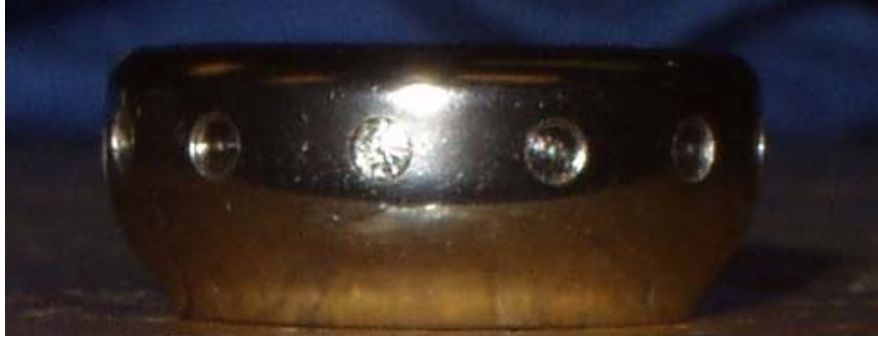
Figure 30: Radial head implant with machined divots.
