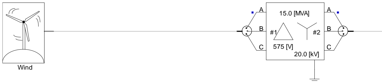
Figure 3.44. Closer look at Wind to the main bus
