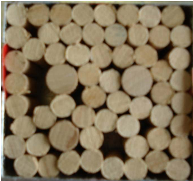
Figure 60. Resulting force chains formed with a 300-lb normal load applied to the seven-millimeter dowel matrix containing 3 nine-millimeter dowels (three dowels were removed).
