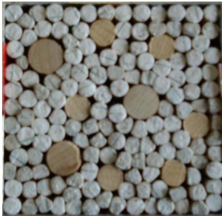
Figure 75. Arrangement of 153 irregular five-millimeter dowels with 3 nine-millimeter dowels and 5 seven-millimeter dowels before applying a 300-lb normal load.
