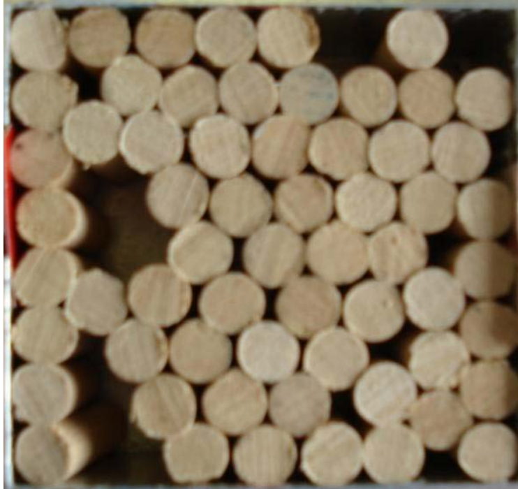
Figure 56. Resulting force chains formed with a 300-lb normal load applied to the seven-millimeter dowels (six dowels were removed).
