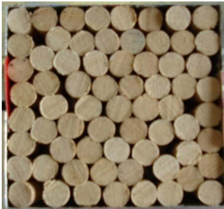
Figure 55. Arrangement of 67 seven-millimeter diameter dowels before applying 300-lb normal load.
