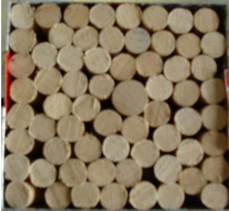
Figure 57. Arrangement of 64 seven-millimeter dowels and one nine-millimeter dowel before applying 300-lb normal load.
