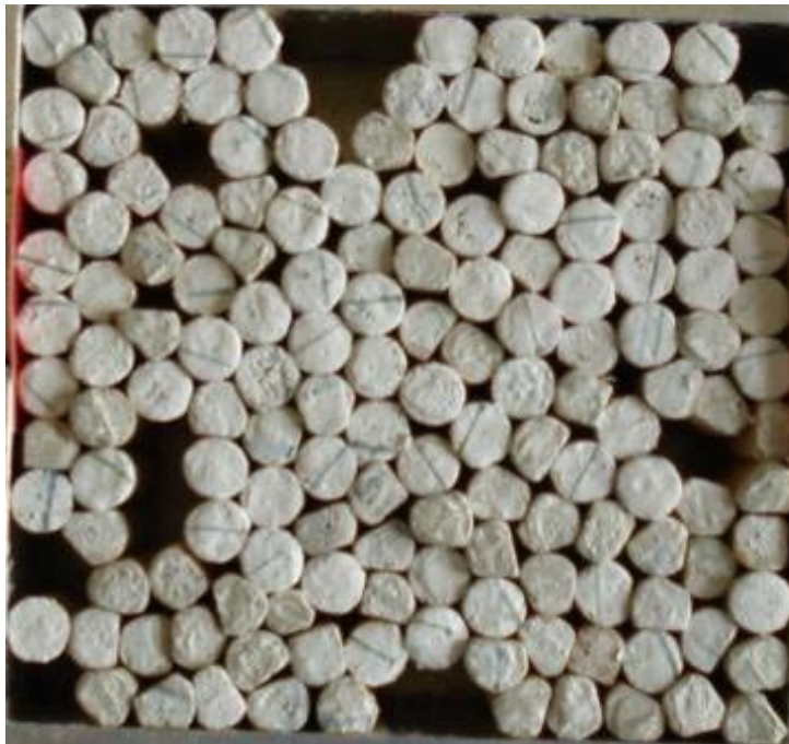
Figure 64. Test A – Force chains developed after applying 300-lb normal load to the irregular five-millimeter diameter dowels.
