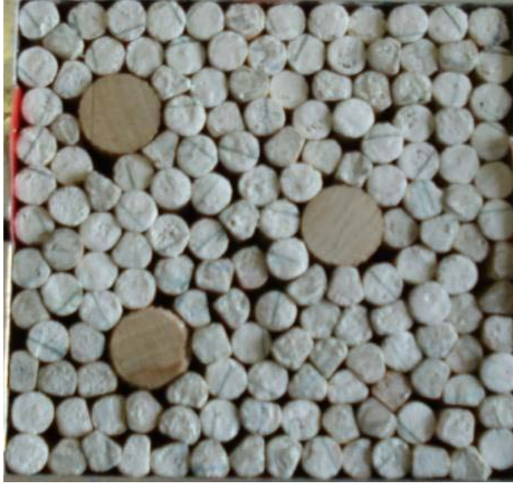
Figure 71. Test C – Arrangement of 159 irregular five-millimeter dowels with 3 nine-millimeter dowels before applying a 300-lb normal load.
