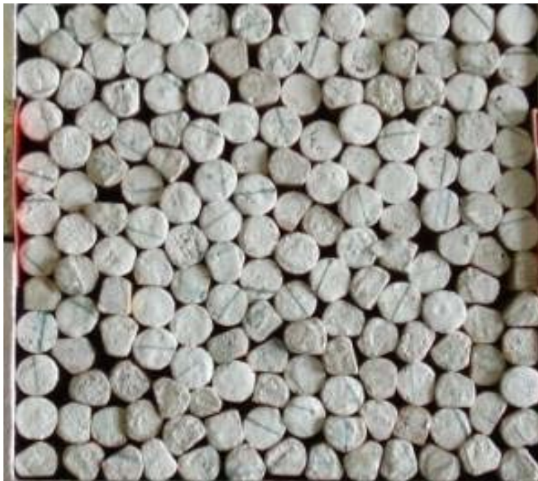
Figure 61. Test A –Arrangement of 164 five-millimeter irregular dowels before applying 400-lb normal load.
