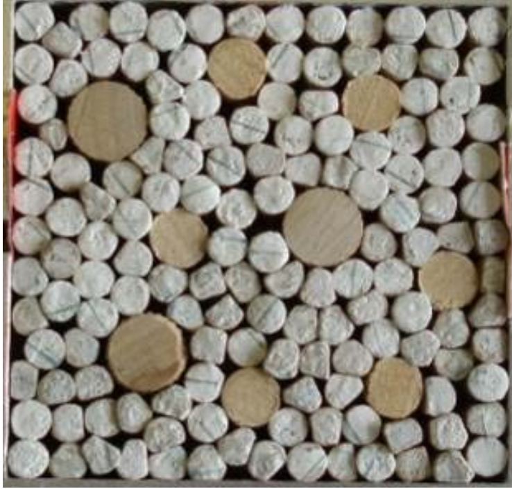
Figure 76. Arrangement of dowels after applying 300-lb normal load – no force chains developed.
