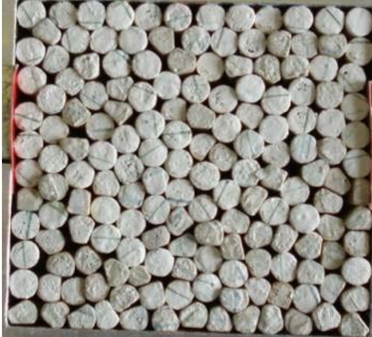
Figure 63. Test A – Arrangement of 164 five-millimeter diameter irregular dowels after applying a 400-lb normal load, before reducing the load to 300 lbs. Note that no arches developed when 400 lbs was applied.
