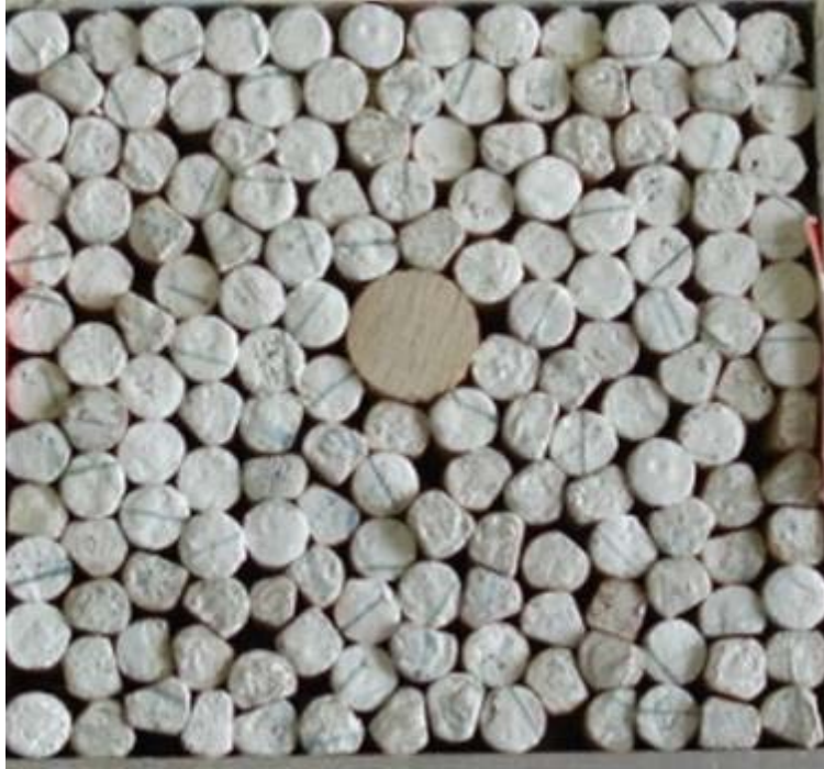
Figure 67. Test B – Arrangement of 159 five-millimeter irregular dowels with a single round nine-millimeter dowel before applying 300-lb normal load.
