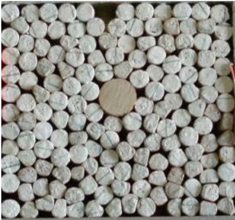
Figure 68. Test B – After applying the 300-lb normal load to the dowel matrix, no force chains developed.
