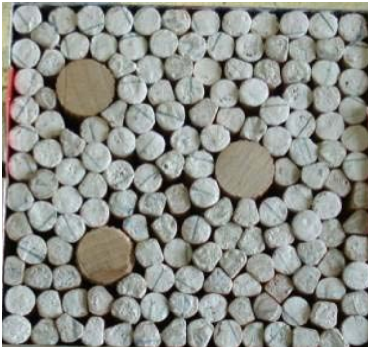
Figure 72. Test C – Arrangement of mixed shape dowels after applying 300-lb normal load. No force chains developed.
