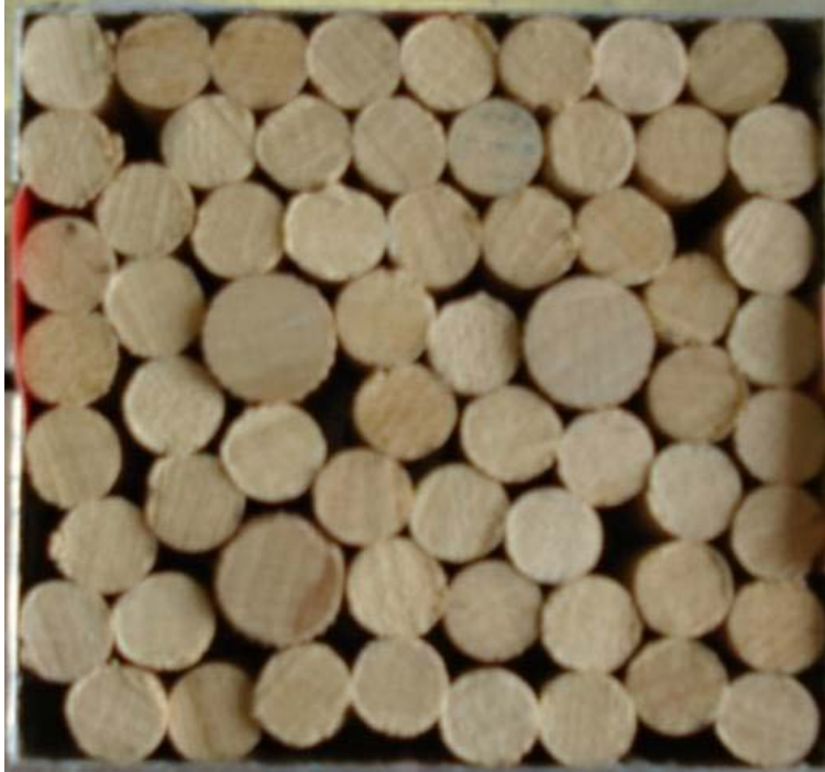
Figure 59. Arrangement of 60 seven-millimeter dowels and 3 nine-millimeter dowel before applying 300-lb normal load.
