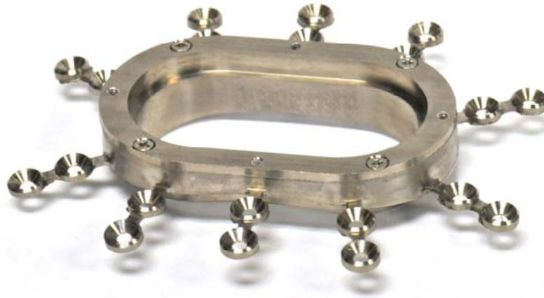
**Figure 32:** Legged recording chamber.
