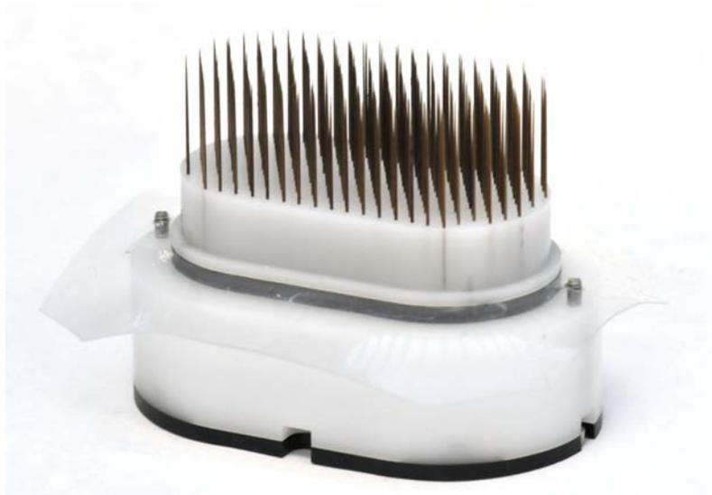
**Figure 39.** Assembled electrode drive, inverted to show fully extended electrodes.
