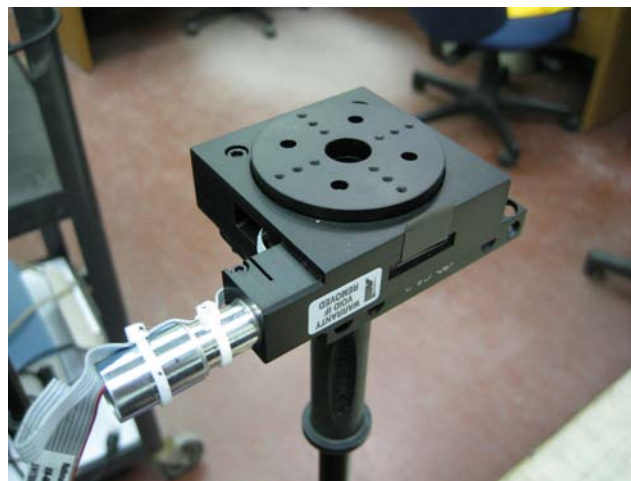
Fig. 7 – Rotational stage controlled by LabView software.
