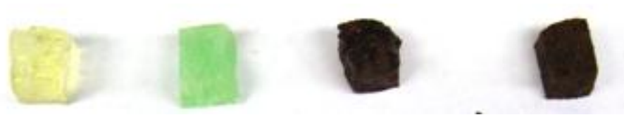
Figure 8. PSS/PA composites components and products: (left to right): PSS/PA hydrogel; PSS/PA hydrogel in polyurethane foam scaffold; PSS/PA hydrogel after FeCl 3 exchange; PSS/PA hydrogel in polyurethane foam scaffold after FeCl 3 exchange.
