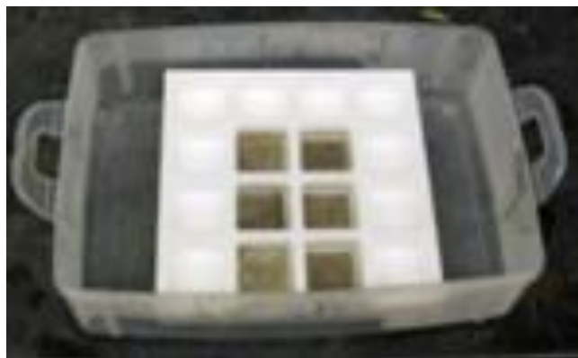
Figure 9. Teflon 16-well plate designed for medium throughput experiments. Six of the sixteen wells contain hydrogel samples.
