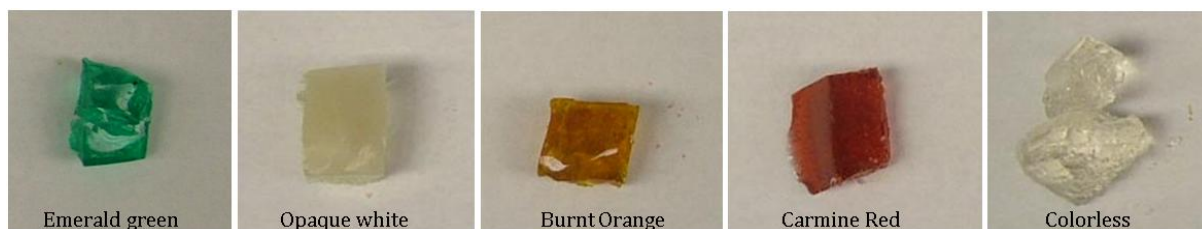
Figure 5. Representative samples of PA/PSS hydrogels with Cu(II), Ba(II), Fe(III), Co(II), and Na(I) (left to right).
