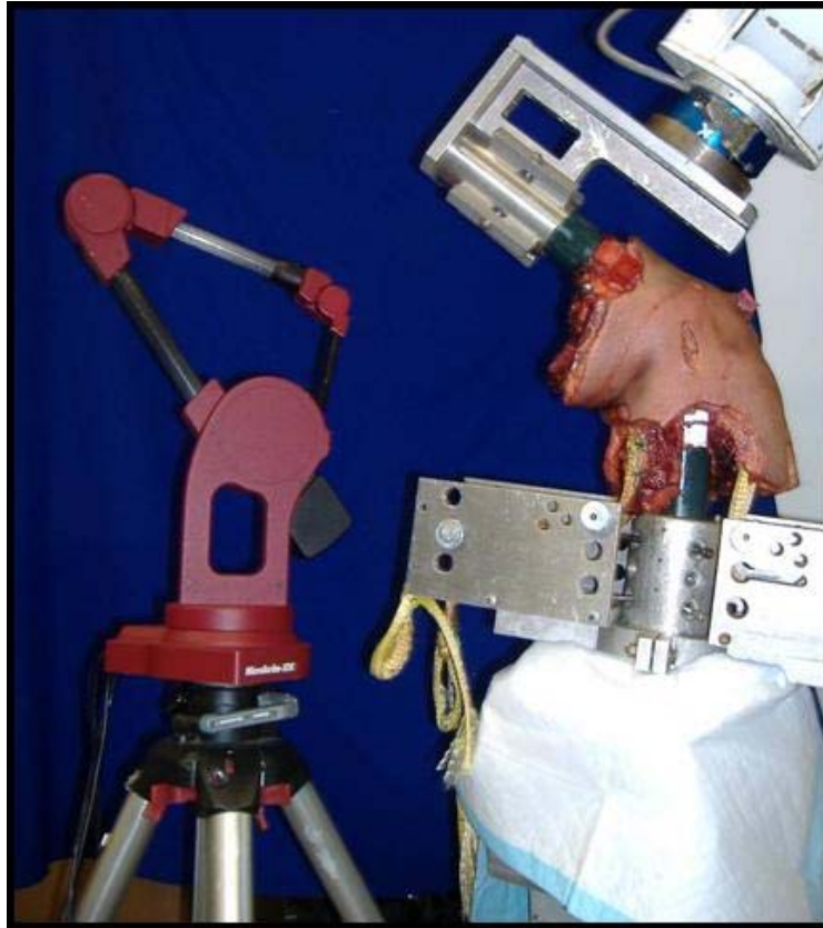
Figure 3-3: Cadaveric knee specimen fixed within robotic/UFS testing system with external digitizer
