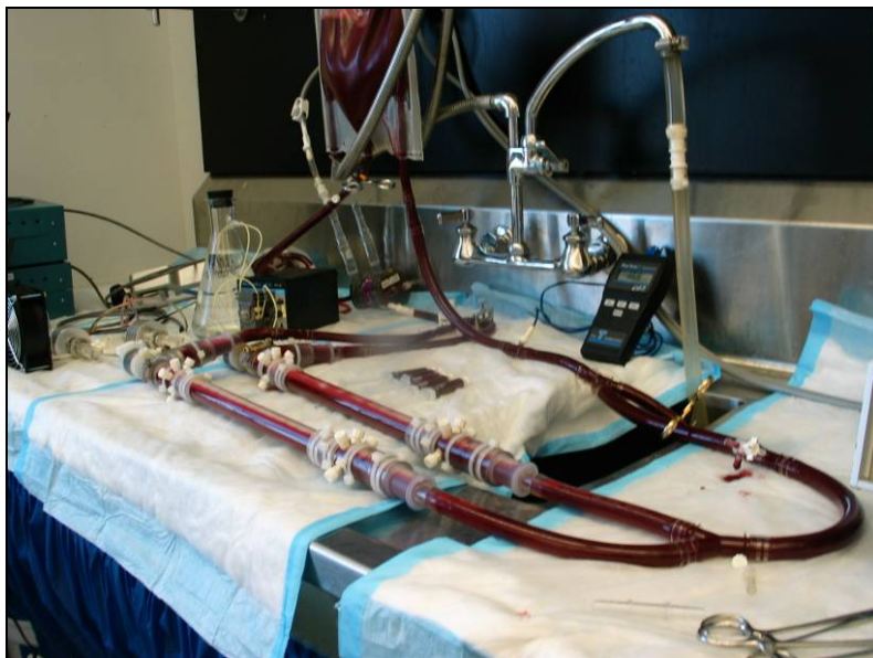
Figure 3-5: Saline purge fatigue test circuit.
