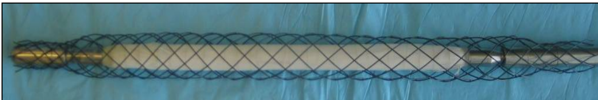
Figure 2-4: RPI-1 nitinol weave safety cage.
