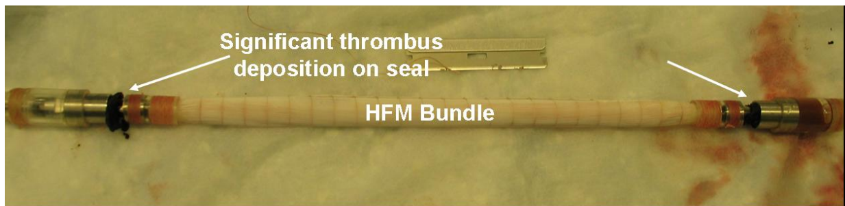
Figure 2-11: Thrombus disparity between RP seals.
