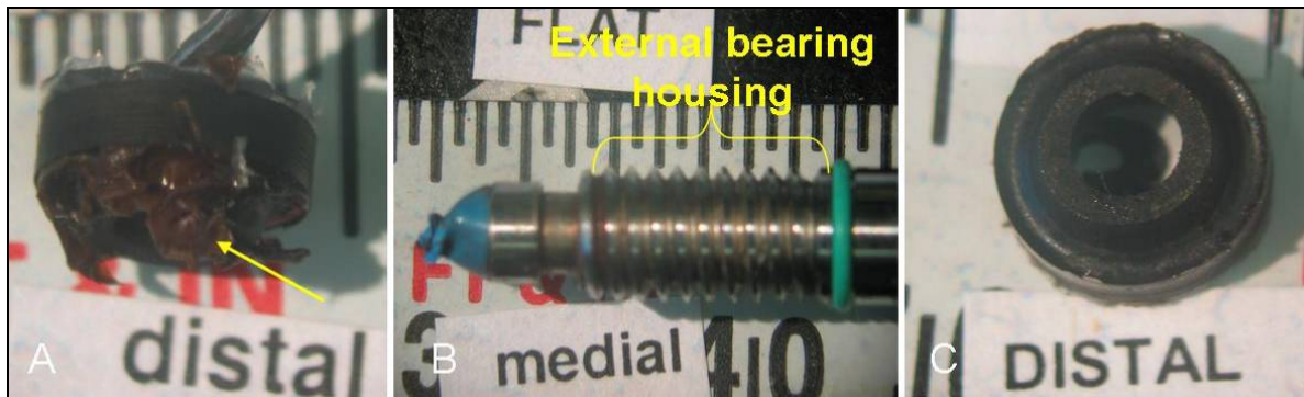
Figure 3-11: (A) Thrombus deposition on seal. (B) External bearing region. (C) Clean seal after successful in vivo operation.
