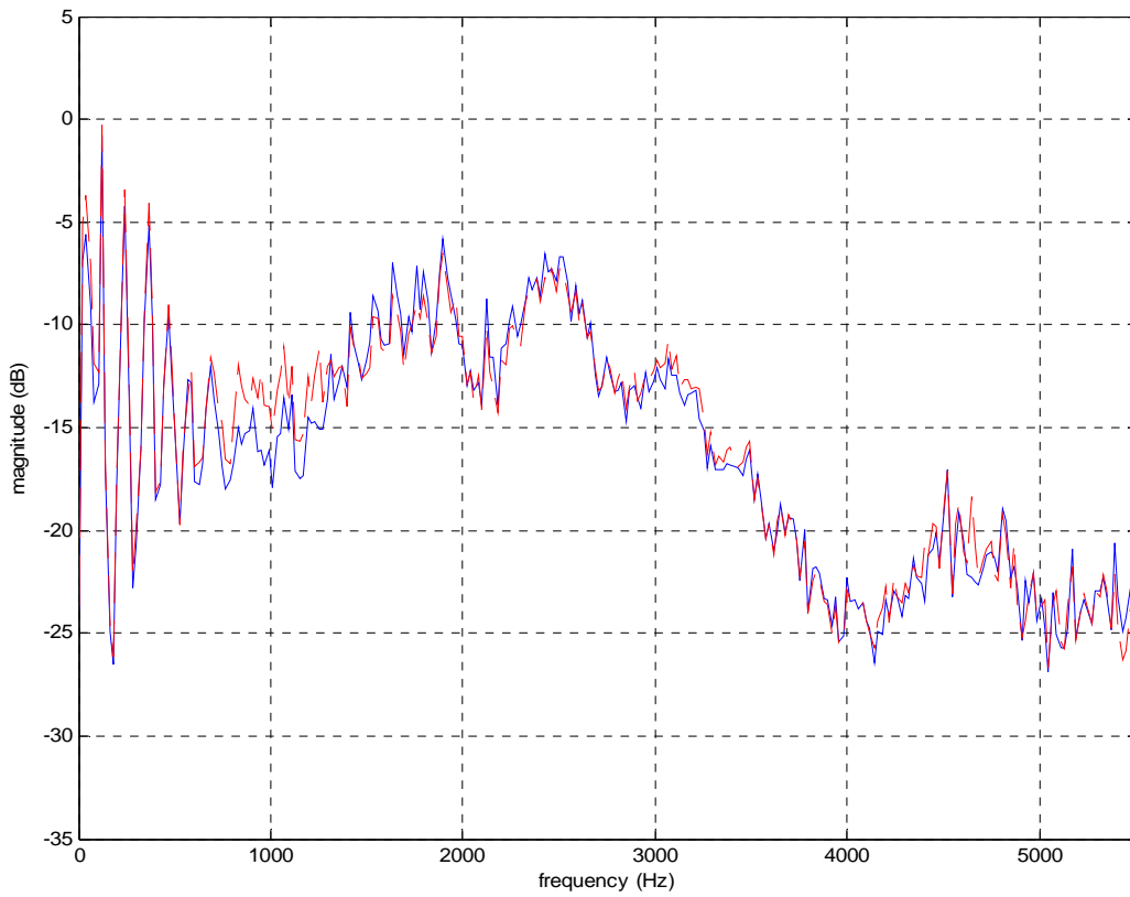
Figure E5: The long-term averaged spectra of enhanced (solid) and pseudo-enhanced (dashed) speech for the F_2(w) - male speaker.
