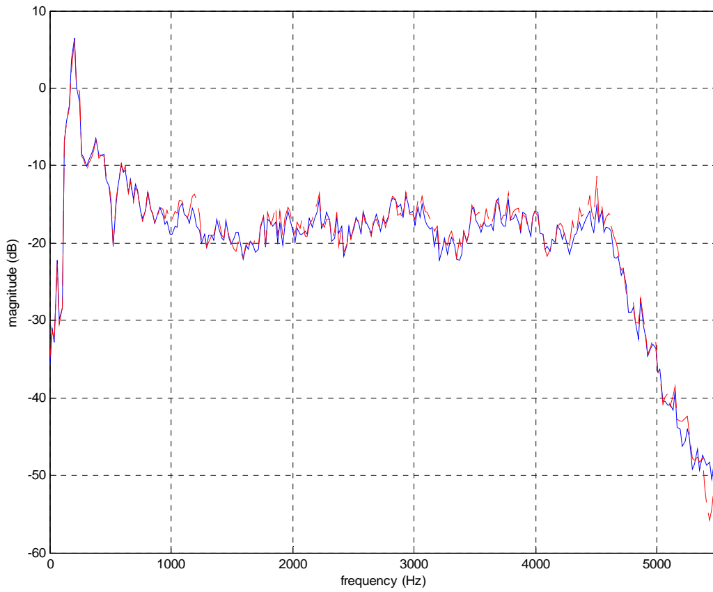
Figure E9: The long-term averaged spectra of enhanced (solid) and pseudo-enhanced (dashed) speech for the F_4(w) - female speaker.
