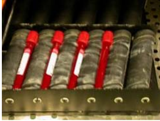
Figure 2-9: Rocker setup for in vitro assessment of materials
