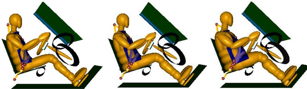
Figure 3-4. Combined Model with BMIs of 25 (Left), 30 (Middle), and 39 (Right).
