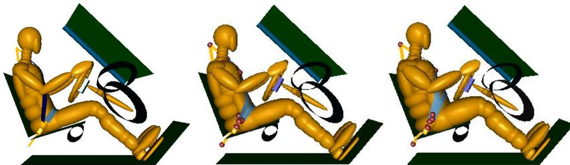
Figure 3-2. Mass Models with a BMI 25 (Left), BMI 30 (Middle), and BMI 39 (Right) in a MADYMO vehicle environment.
