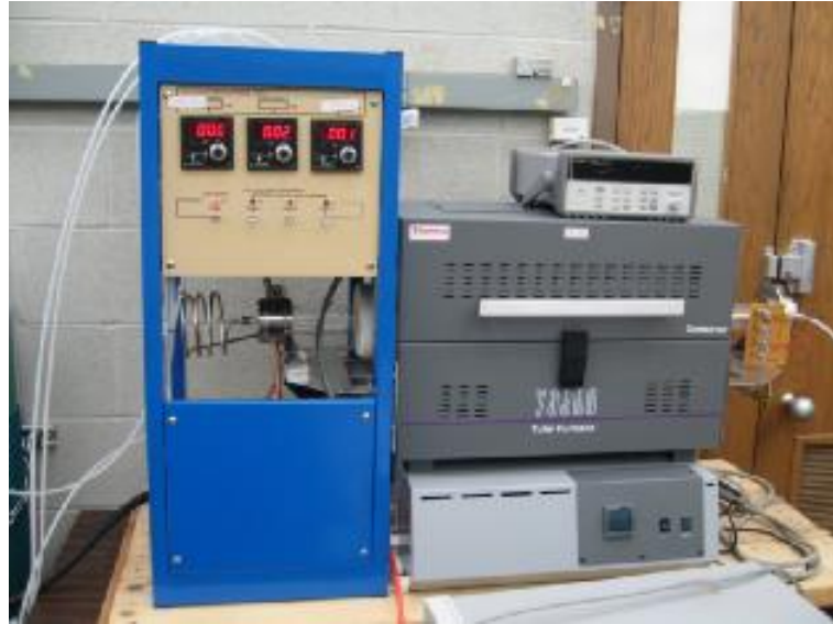
Figure 4.7. Custom CVD 200M system
