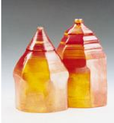
Figure 4.1. Langasite (LGS) crystal
